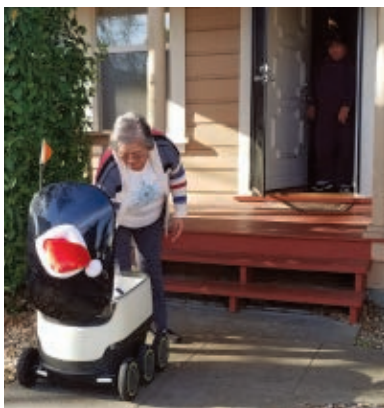
Starship Technologies' six-wheeled delivery robot is 27 inches long by 22 inches wide and can carry up to 20 pounds within a two-mile radius. This one delivered holiday gifts to residents of Redwood City, California, where the European company has an office.
