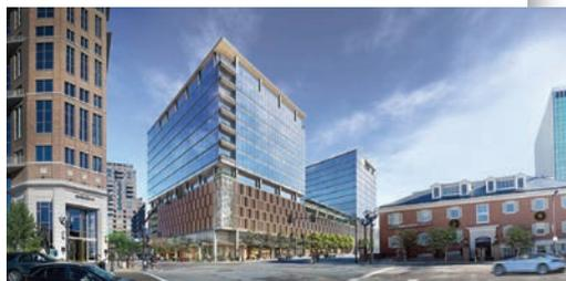
includes two Class A office towers with 20,000 square feet of street-level retail space. The steel-framed glass structures rest atop a post-tensioned concrete-framed seven-level parking structure. At the top level of the parking structure, a 45,000-square-foot open-air garden terrace will serve as a signature amenity and be available for public events. The project is expected to be completed in the summer of 2022.
