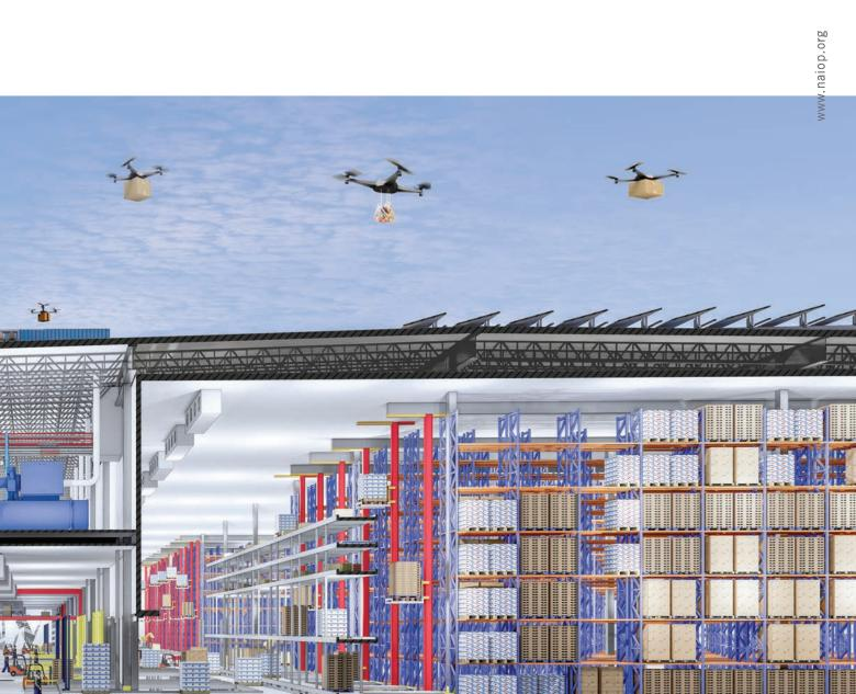
A section view of a cold-ready building showing refrigerated storage, the cold dock and the equipment mezzanine.
