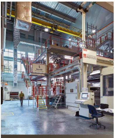
This nonwoven spunbond extruder machine occupies the first floor of the Center for Technology & Innovation. It's used by N.C. State's Nonwovens Institute (NWI), a partnership between industry, government and academia that's affiliated with the N.C. State College of Textiles. The machine, which is roughly 52 feet tall and 170 feet long, produces prototypes of fabrics that are used in a variety of consumer, medical and industrial applications.
